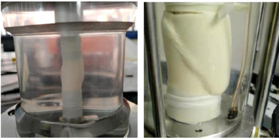
Fig. 4 Contrast tests between miniature triaxial apparatus and conventional triaxial apparatus
