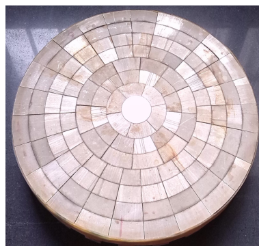
图 3 岩土工程三轴试验微摩擦荷载传力板实物照片 Fig. 3 Physical photo of load-transfer plate under micro-friction in triaxial tests in geotechnical engineering
