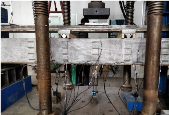
图 6 钢-SCC 组合梁试验 Fig. 6 Tests on steel-SCC composite beam
