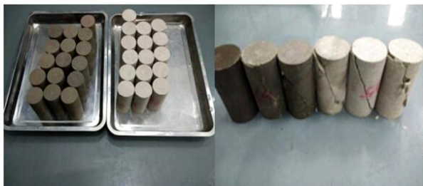
图 2 干燥、饱和砂岩试样及其破坏 Fig. 2 Dry and saturated sandstone samples and their failure
