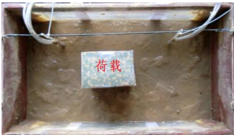
图 6 振动前模型试样 Fig. 6 Model of sample before shaking
