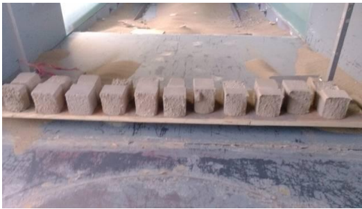
(a) 风蚀后试样形态
