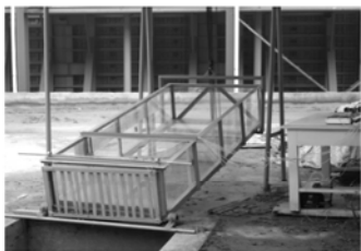
图 4 蠕滑模型槽实物图 Fig. 4 Schematic description of set-up of model
