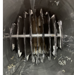
图 6 块石定向性实现装置 Fig. 6 The device for realizing rock block orientation features
