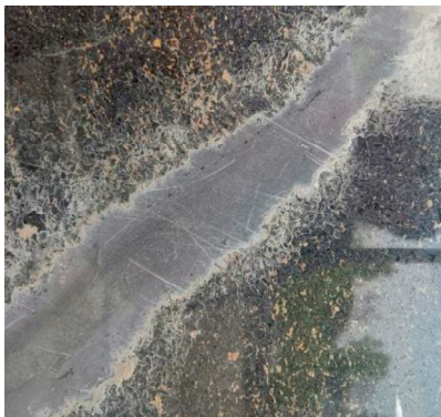
图 8 试验形成的注浆体 Fig. 8 Grout formed by tests
