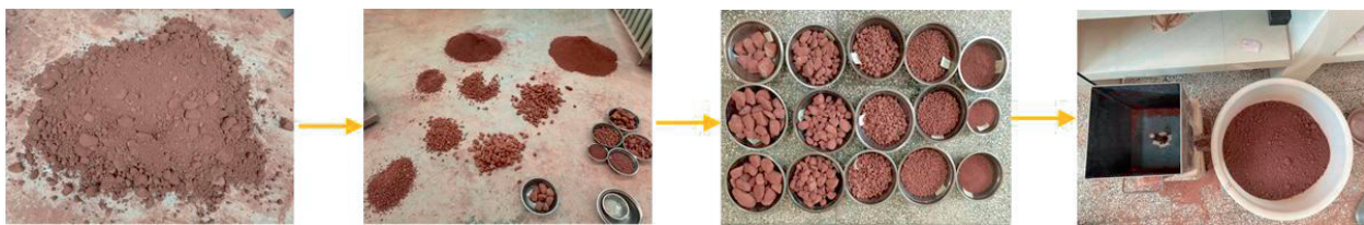
图 14 全级配砾石土含水率快速检测验证试验 Fig. 14 Quick detection tests on moisture content of fully grade gravel soil
