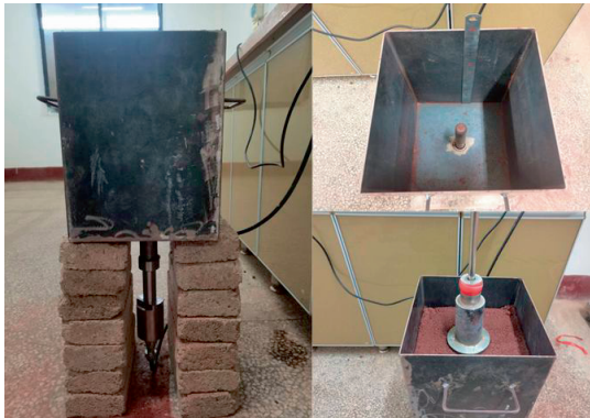
图 10 标定装置结构及制样方式 Fig. 10 Structure of calibration devices and preparation method for sample
