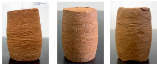
图 7 非饱和三轴压缩试验结束后的试样 Fig. 7 Soil specimens after unsaturated triaxial compression tests
