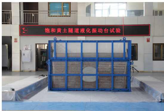
图 3 饱和黄土隧道振动台试验 Fig. 3 Shaking-table tests of saturated loess tunnel
