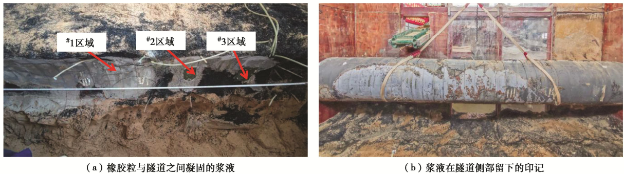
Fig. 13 Corresponding development of different slurry diffusion modes
