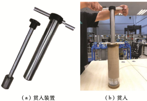
Fig. 2 Scheme of set-up for infiltration tests
