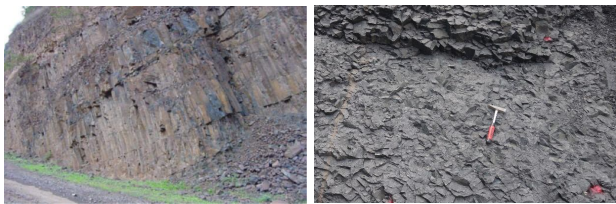
图 2 白鹤滩水电站第一类柱状节理玄武岩典型照片 Fig. 2 Typical photos of the first type of columnar jointed basalt in Baihetan Hydropower Station
