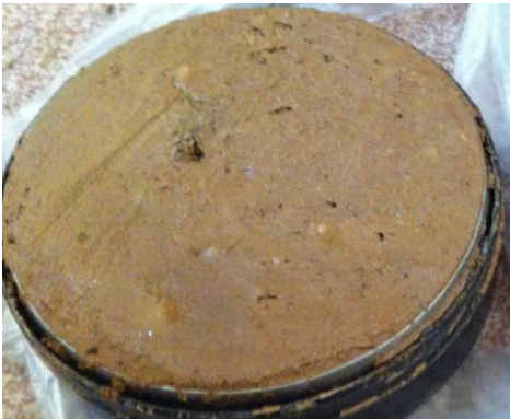
图 14 自然气候长期服役有植被条件下覆盖层红黏土结构 Fig. 14 Structure of red clay cover with vegetation in long-term service in natural climate
