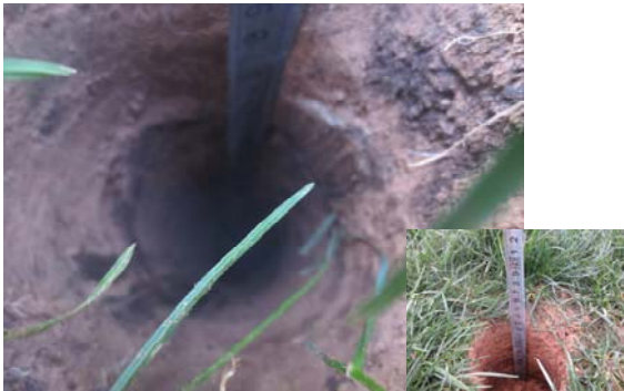
图 19 长期服役过程中现场探洞观测有植被条件红黏土裂缝 Fig. 19 Observation of cracks in red clay with vegetation by on-site exploration during long-term service
