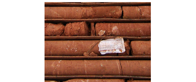
图 2 成都地区典型中等风化泥岩岩芯 Fig. 2 Typical moderately weathered mudstone core in Chengdu
