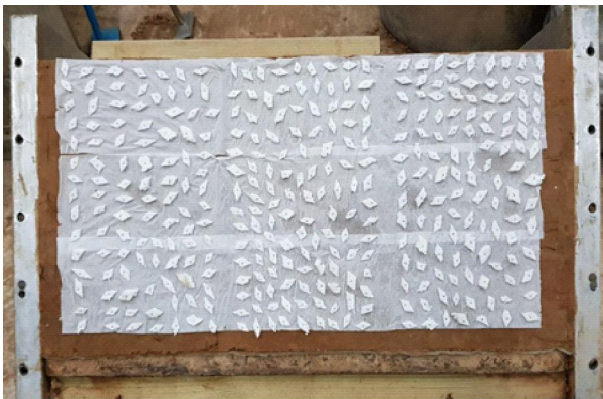
图 4 天然含水率土样模型 Fig. 4 Model made of soil with natural moisture content
