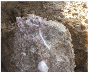
图 1 五彩湾试验场地粗颗粒盐渍土地层断面 Fig. 1 Strata of coarse-grained salty soils in Wucai Bay
