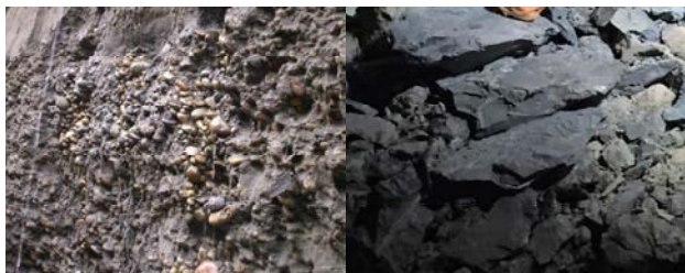
图 2 典型圆砾地层(左)与泥岩地层(右) Fig. 2 Round gravel (left) and mudstone (right)
