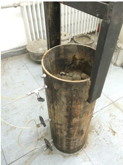
图 4 填装渣土的试验桶 Fig. 4 Barrel for testing permeability of conditioned muck
