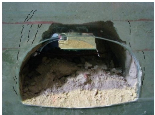
(e) 左、右侧拱肩及拱顶继续塌落, \Delta P = 17.68 kPa
