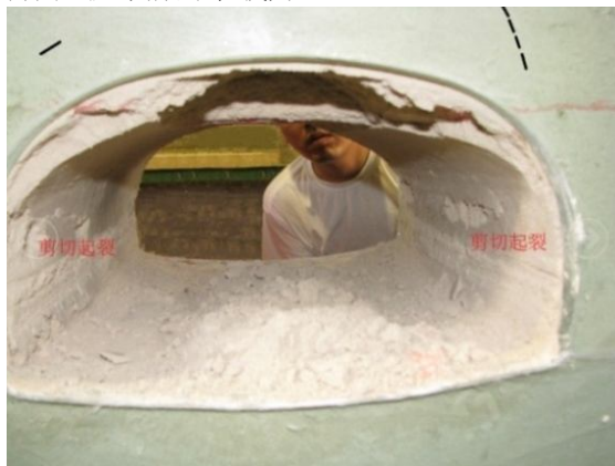
(a) 拱腰剪切起裂、拱顶出现裂缝, \Delta P = 10.37 kPa
