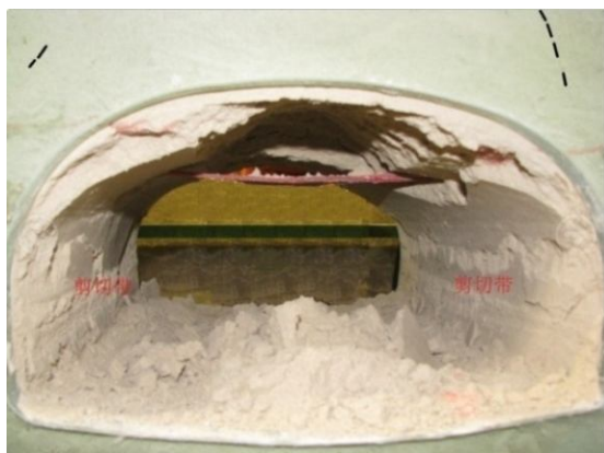
(b) 拱顶、拱腰进一步塌落, \Delta P = 11.99 kPa
