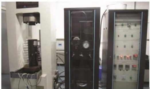
图 1 TAW-2000 型电液伺服岩石力学试验系统 Fig. 1 TAW-2000 electro-hydraulic servo rock mechanical experimental system
