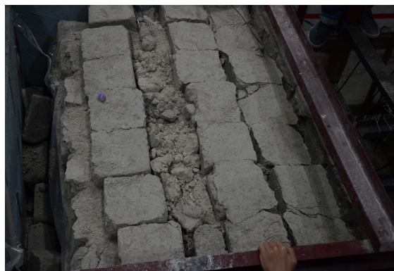
(c) 坡顶张拉裂隙, 后缘分离
