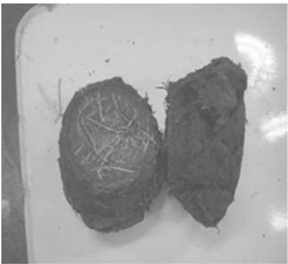
图 7 K0+600 断面试样无侧限抗压强度试验后 Fig. 7 Sample at K0+600 after unconfined compressive strength tests
