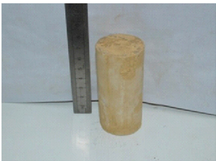
图 1 黏土-石膏胶结试样 Fig. 1 Cementation sample of clay-gypsum cementation
