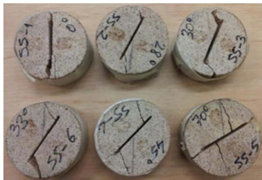
图 7 CCNBD 复合型断裂试验破坏结果 (引自文献[9]) Fig. 7 Realistic mixed mode fracture failure of CCNBD (from Ref. [9])
