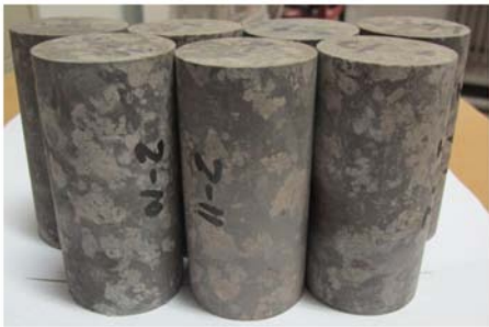
图 1 制备得到的泥质粉砂岩试样 Fig. 1 Argillaceous siltstone specimens for stress relaxation tests
