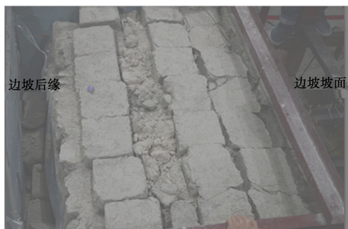
(b) 坡顶张拉裂隙,后缘分离
