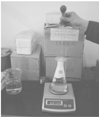
Fig. 3 Volume of EPS beads measured by drainage method
